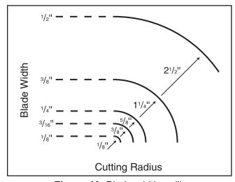
Figure 46. Blade width radii.
